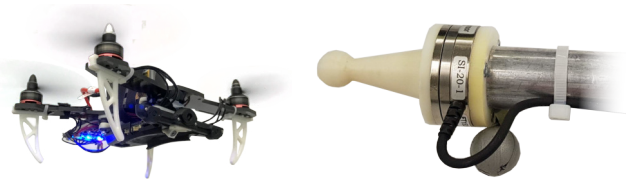
(a) Snapdragon Flight Quadrotor (b) Force sensor ATI Mini40 Fig. 6: Experimental quadrotor platform (a) and an force/torque sensor (b).
