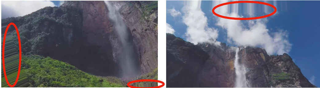
Figure 13: Typical visual artifacts when the rendering viewpoint moves out of the currently available VAM frame
