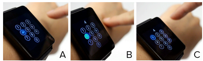
Figure 12. The back of the hand can be used as a number keypad. Finger hover location controls an on-screen cursor (A,C) to assist in targeting buttons (B).
