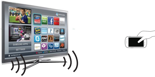
Figure 1: Enabling accurate device tracking using the Doppler effect of the acoustic signal.
